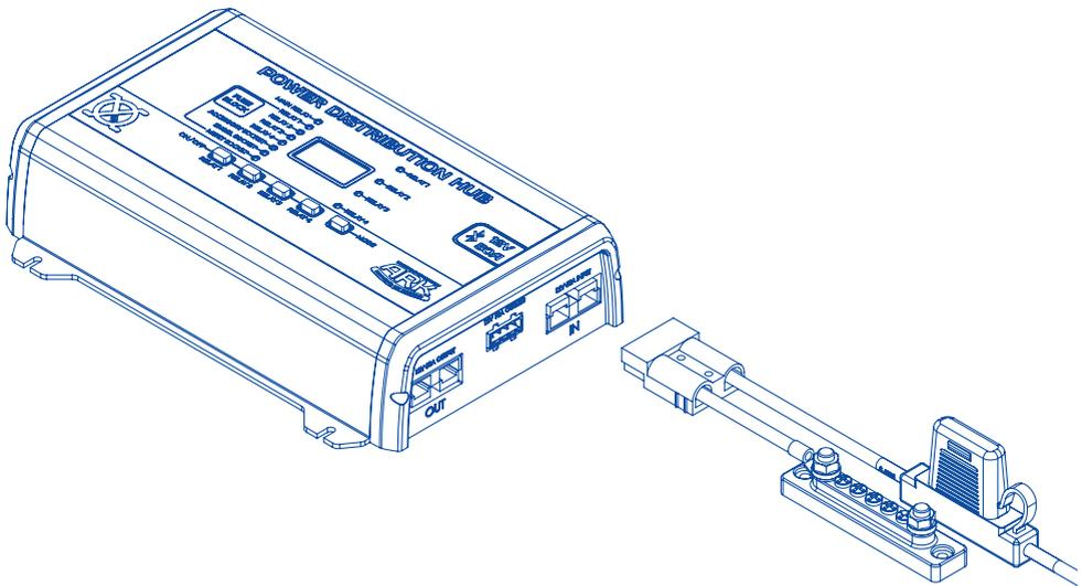
**HANDY HINT** - Using a negative busbar will prevent the need of returning all your negative lines from your devices controlled by the 4 x Relay outputs back to the battery and provide a common ground for these devices.
