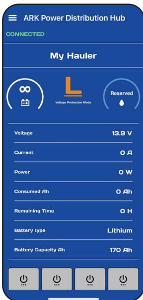
The PDH has a smart feature to detect when your battery is being charged as explained in Section 4.3. When the PDH detects the battery is being charged, the battery status section will change to “∞”.
