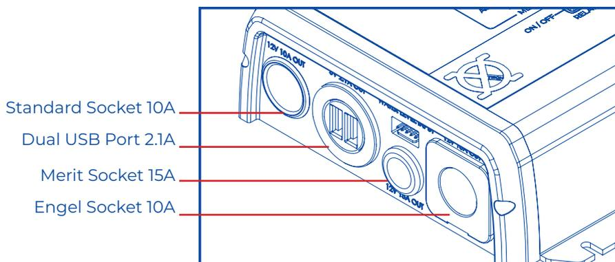
**CAUTION** - If all outputs are used at once, the total maximum current the PDH can operate is 50A only, if overloaded the device will enter Current Protection Mode (Page 9)
