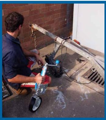
A jockey wheel is a great, affordable addition to any trailer. Before you attach the new jockey wheel, remove any wiring and brackets that are in the way. Find a suitable position that won't interfere with the winch post or trailer hitch.
