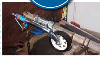
With the mounting plate loosely attached to the drawbar, operate the jockey wheel through its full range of motion to check for clearance of the hitch point and the winch post. In my case I had to move the mounting plate back around two inches.
