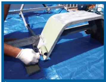
★ To bring the trailer back to life, it's time for a coat of paint. There are a few different methods you can employ, for example spraying or rolling, Killrust™ offers pressure packs or paint tins – I opted for the paint tin and roller. After you have prepared the surface and wiped it with wax and grease remover, it's time to roll on the paint. Make sure you don't go overboard as too much paint will cause runs.
