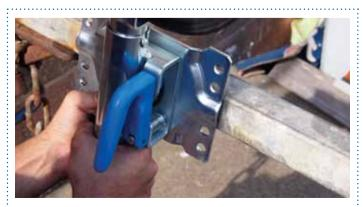
Hold the jockey wheel vertically in the rough location it is to be fastened (my trailer is upside down, due to the total rebuild). Align the holes in the mounting plate with the draw bar and insert two U-bolts surrounding the draw bar in the process.
