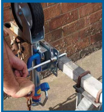
Once you're happy with the location of the mounting plate, tighten the four bolts so that they are nice and firm. Operate the wheel through the full range of motion again and check for clearance. Mark where the mounting plate is so that when you remove it for painting, you know exactly where it needs to be.
