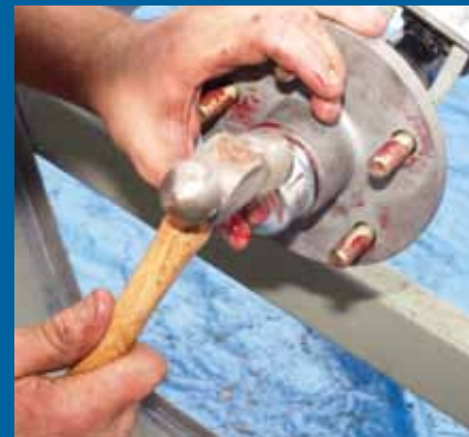
The last stage of the hub is the dust cap. No need to panel beat this into place – just a light tap around the edge and it will fall into place.
