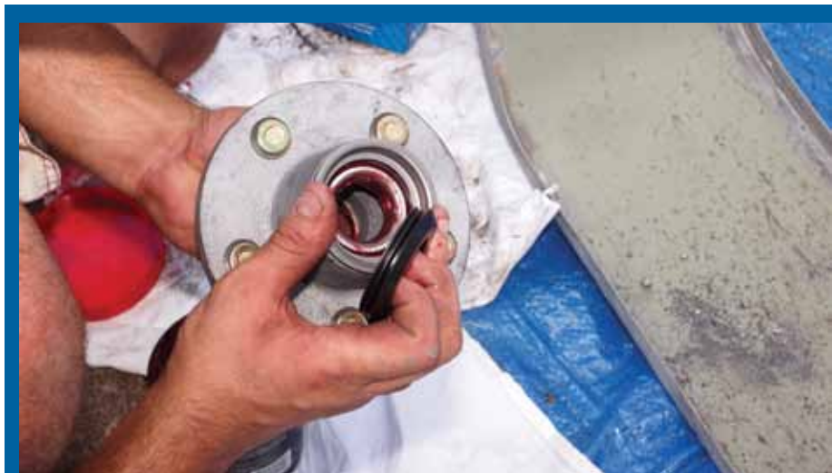
Once you have packed all bearings with grease, it's time to assemble the hub. Place the inner bearings in first (the bearings will only go in one way), followed by the waterproof rubber seal then simply turn over and put the outer bearing in.
