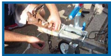
(I'm replacing the hitch as well as the old one is fairly worn. If you don't have a jockey wheel, the hardware here can be very stubborn to replace as this is where the trailer cops most of its punishment. In my case I had the grinder handy which made light work of the bolts.
