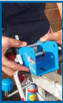
Now to line up the new winch. Mark a centre line where the winch is going to sit — hopefully the holes from the old winch line up with the new one. If only one lines up like it did for me, put the new bolt through the hole and tighten it up just enough so the winch can just move. Make it as straight as possible and mark out the new hole with the drill.
