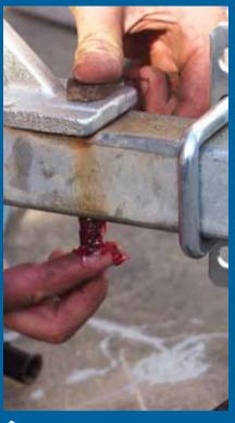
Simply clean back the surface of the trailer so it sits true, then it's just a matter of putting the new bolts through and tightening them up.
