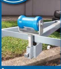
To obtain the right height of the rollers, you want to have a starting point. Firstly, install all rollers, adjusting them enough that the boat will clear the wheel arches and be as level as possible.
