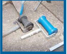
Two of the fastest wearing parts on your trailer are the rollers and skids, which bear the brunt of the punishment from the salt and the sun's UV rays. The polyurethane starts to break down after years of harsh treatment making it difficult to selflaunch and recover your boat.
