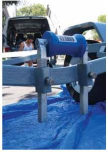
At the rear of the trailer, the same principle applies. The centre roller has two adjustments try to keep them even or irregular wear will occur.
