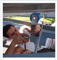
This is the same for the rest of the rollers and skids. To reduce your boat from thumping around on the trailer while driving, have about an inch gap between the boat and the wheel arches. If the boat needs lifting in places, the easiest way I have found is to utilise a car jack and some pieces of timber – it beats trying to lift it yourself.
