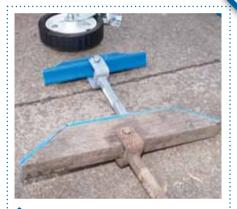
You'll find many of the older trailers will have bulky timber skids. Yes these are larger than the new lightweight ARK polyurethane skids, as well as being twice the weight. They also tend to wear a lot faster, preventing them from moving freely.
