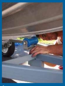
Now to make those rollers work! The easiest way to do this is to load the boat back onto the trailer with the aid of a mate. Lie underneath the boat and slide the rollers up to meet the bottom of the hull - make sure you keep the rollers straight.
